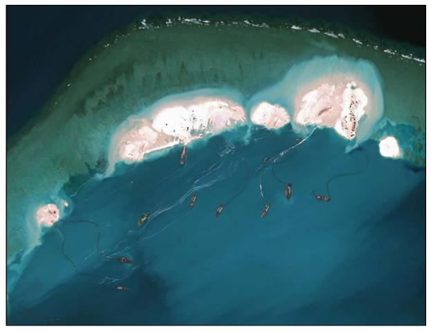
Figure 17: Dredgers at work at Mischief Reef (Annex 792)
