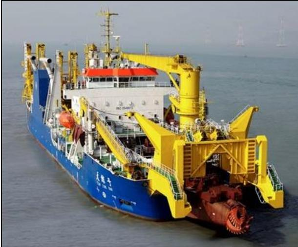
*Figure 15: Tian Jing Hao, Cutter-Suction Dredge
