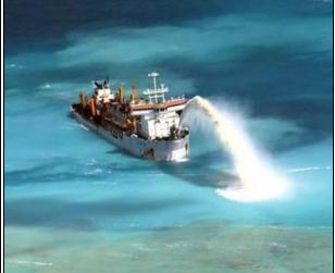
Figure 16: Trailing Suction Hopper Dredge (Annex 792)
